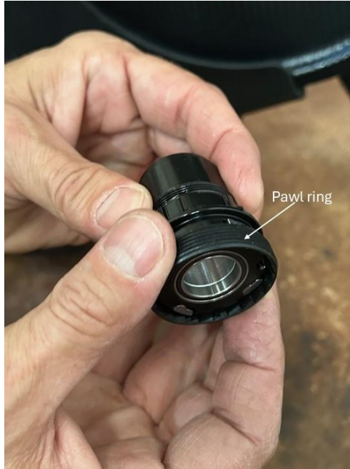
6. Remove the pawl ring from XDR Body
