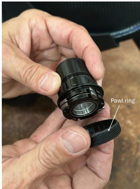
7. Pawl ring not required on the Victory
